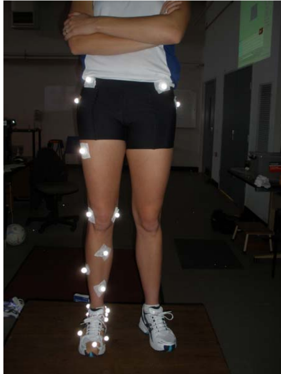
Figure 2: Markers attached to the shoe, and on the foot, shank, thigh and pelvis.
