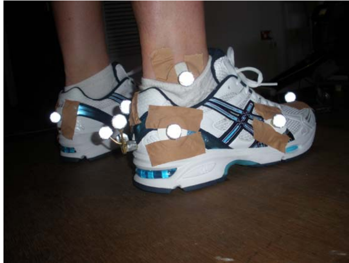
Figure 3: The rearfoot wand and the markers on the shoe.
